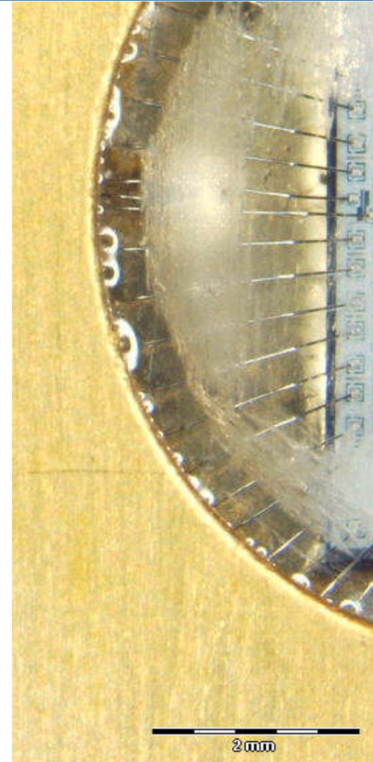
Scratched Window from Sanding and Corroded Metal
