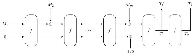
Figure 3.7: PHOTON-Beetle-Hash with  $m$  message blocks. Here  $|M_1| = 128$ ,  $|M_i| = r$ , for  $i = 2, \dots, m - 1$  and  $|M_m| \leq r$ . The tag  $T$  is computed as  $T_1^* || T_2^*$ , where  $T_i^* = \text{Trunc}(T_i, 128)$ .
