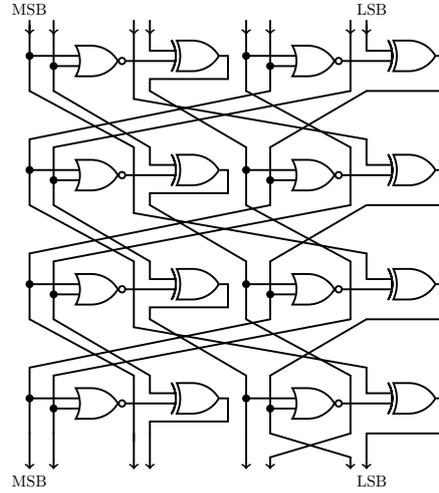
**Figure 2.2:** Construction of the Sbox  $\mathcal{S}_8$ .
