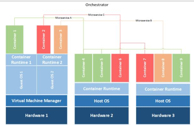
Figure 5: Container Technology Stack
