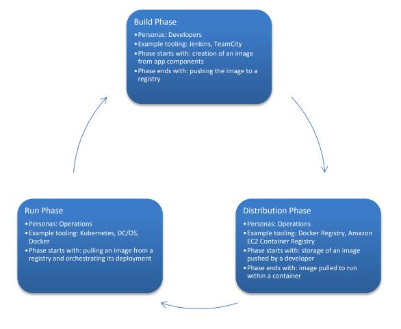
Figure 4: Container Lifecycle Phases
