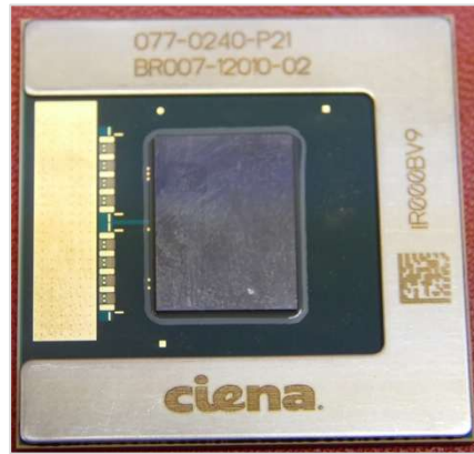
Figure 2: SoC in which the entropy source is implemented.
