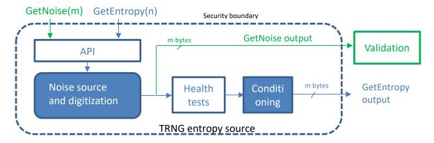
The TRNG (inside its security boundary) is composed of:
