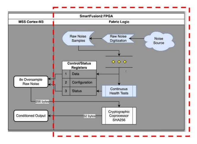
The security boundary of the CTC entropy source surrounds the Fabric Logic as seen in the figure above. This boundary includes the entropy source, the digitization, the health tests, and the conditioning function.
