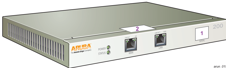
Figure 3-12 Required TELs for the Aruba 200 Mobility Controller
