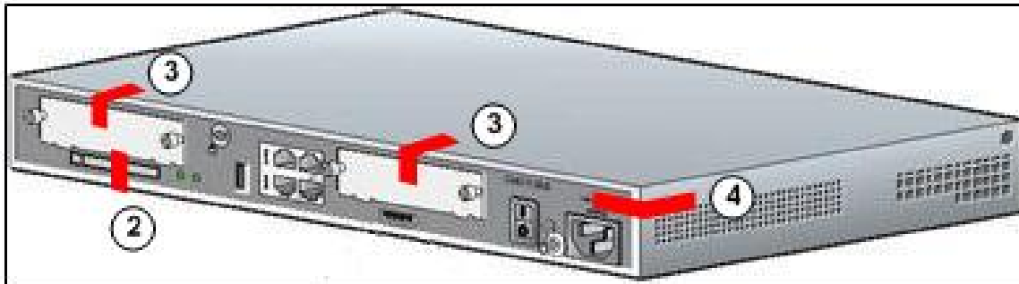
Figure 11 – Cisco 1841 Tamper Evident Label Placement (Back View)
