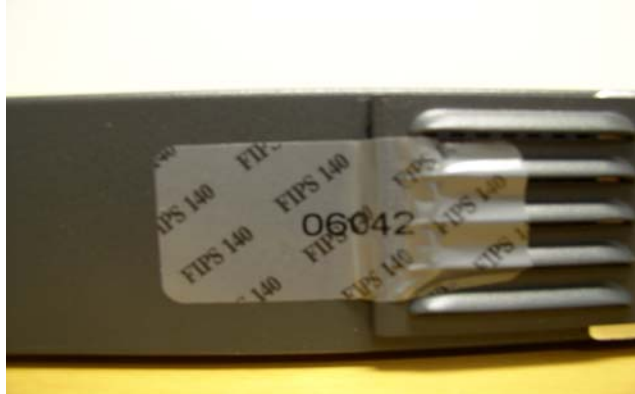
Figure 6 Tamper evident labels attached on the opacity shield of Router 1841
