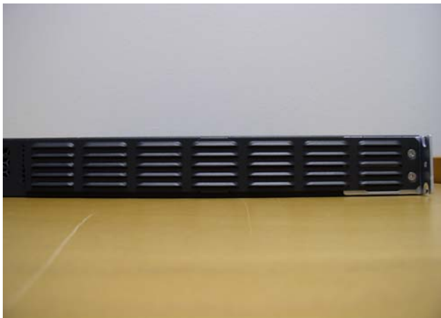
Figure 8 Opacity shield attached on the side panel of router 2801
