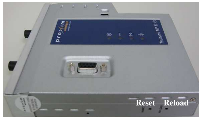
Figure 7 – Tsunami MP.11 HS 245054_S Buttons
