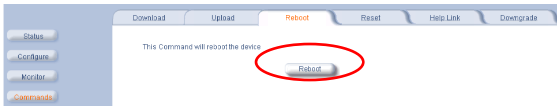
Figure 9 – Rebooting the Device on Web Interface
