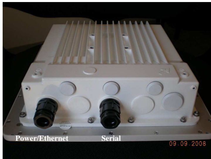
Figure 2 – Tsunami MP.11 HS 245054_R Ports
