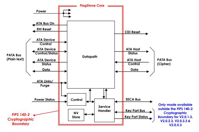
Figure 8 - FlagStone Core Simplified Block Diagram
