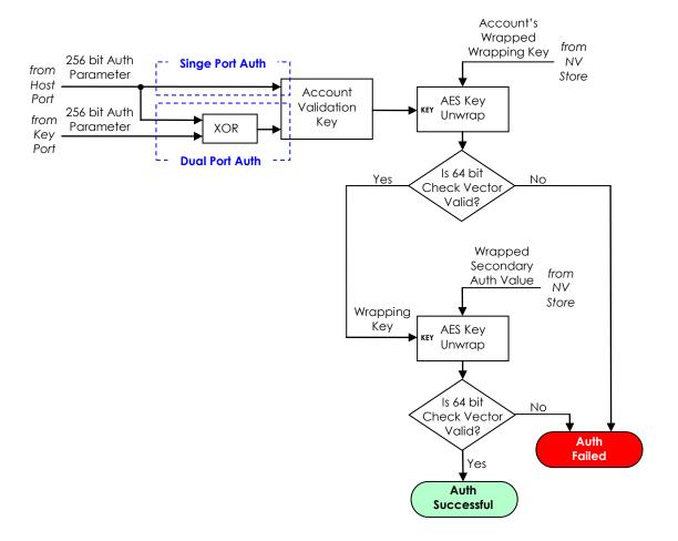
Figure 10 - Authentication Mechanism
