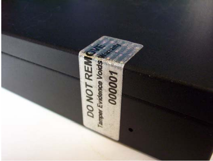
Figure 3: Tamper evident seal on the rear of the CEP10-R chassis
