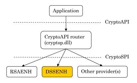
Figure 2 Relationship to other components in Windows CryptoAPI system – cryptographic module shown in gold
