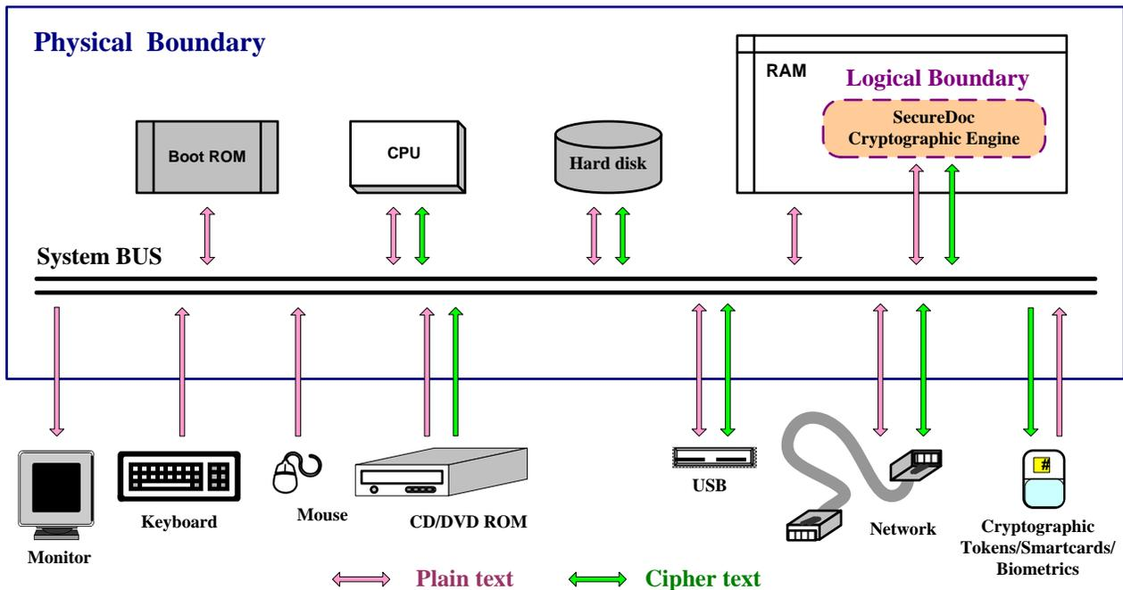
Figure 1 - Cryptographic Module Block-Diagram
