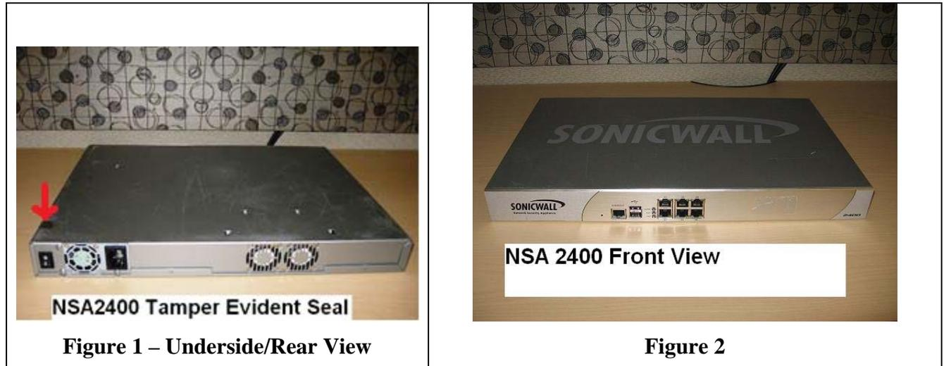
The tamper evident seal is applied by SonicWALL during the manufacturing process. The Cryptographic Officer should inspect the module to ensure that the tamper evident seal has been applied on the bottom of the module, as shown above. The Cryptographic Officer must physically inspect the module for signs of tamper every six months. If the module shows any evidence of tamper, the Cryptographic Officer should contact SonicWALL, Inc.
