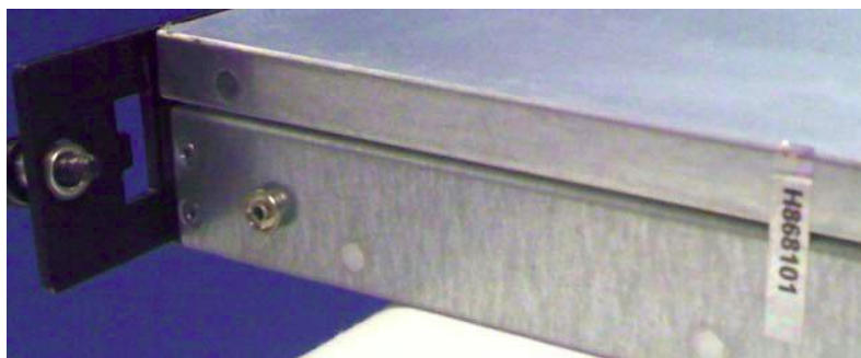
Figure 5 – Tamper-Evident Label Placement (Chassis/Cover - right)
