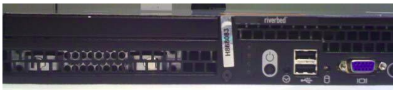
Figure 7 – Tamper-Evident Label Placement (Faceplate)
