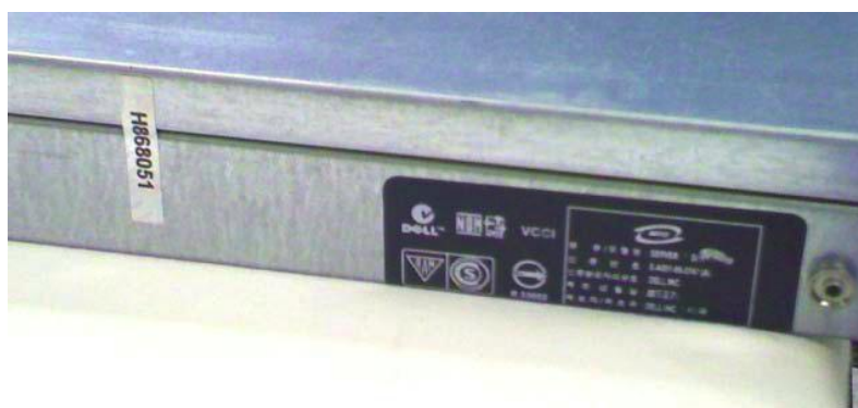
Figure 6 – Tamper-Evident Label Placement (Chassis/Cover - left)
