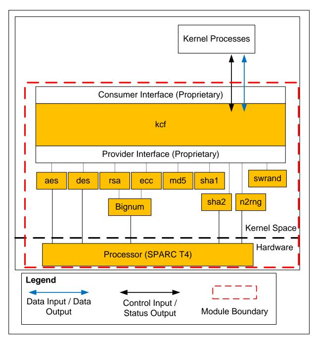
Figure 1 - Oracle Solaris Kernel Cryptographic Framework with SPARC T4 and T5 Logical Block Diagram  $-\,\text{T4}$
