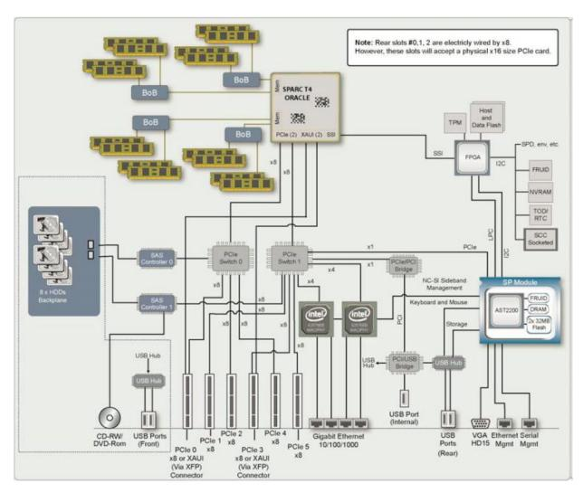
Figure 3 – T4-1 Server Hardware Block Diagram
