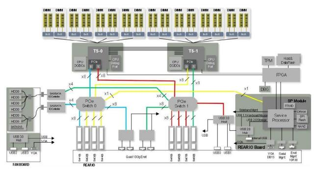
Figure 4 – T5-2 Server Hardware Block Diagram
