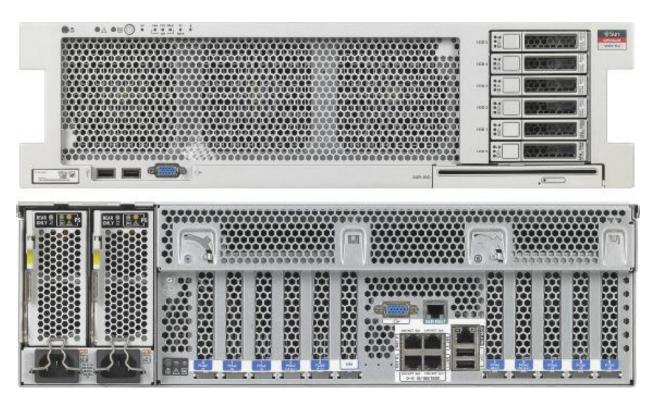
Figure 8 – T5-2 Server Front and Rear Ports (SPARC T5-based)
