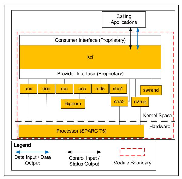
Figure 2 –Oracle Solaris Kernel Cryptographic Framework with SPARC T4 and T5 Logical Block Diagram – T5
