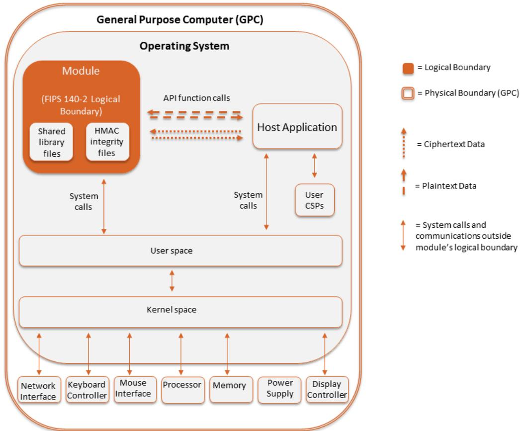
**Figure 1 – Module Boundary and Interfaces Diagram**
