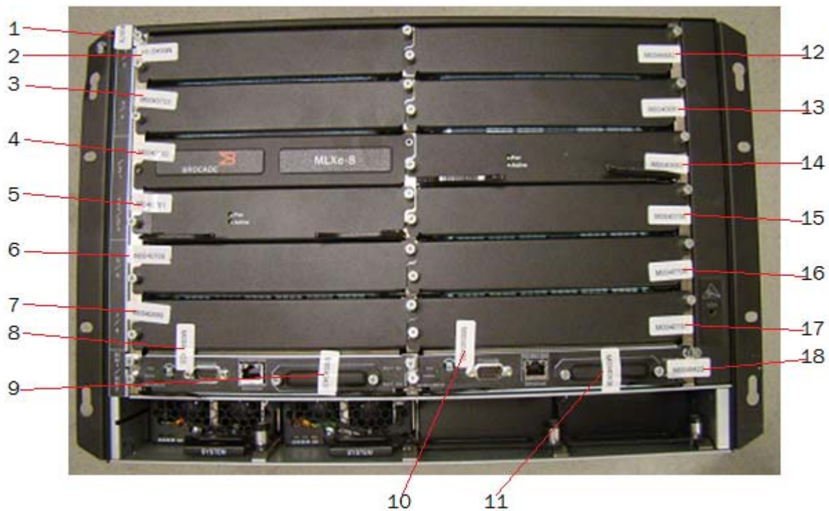
Figure 15 Front view of a Brocade MLXe-8 device with security seals
