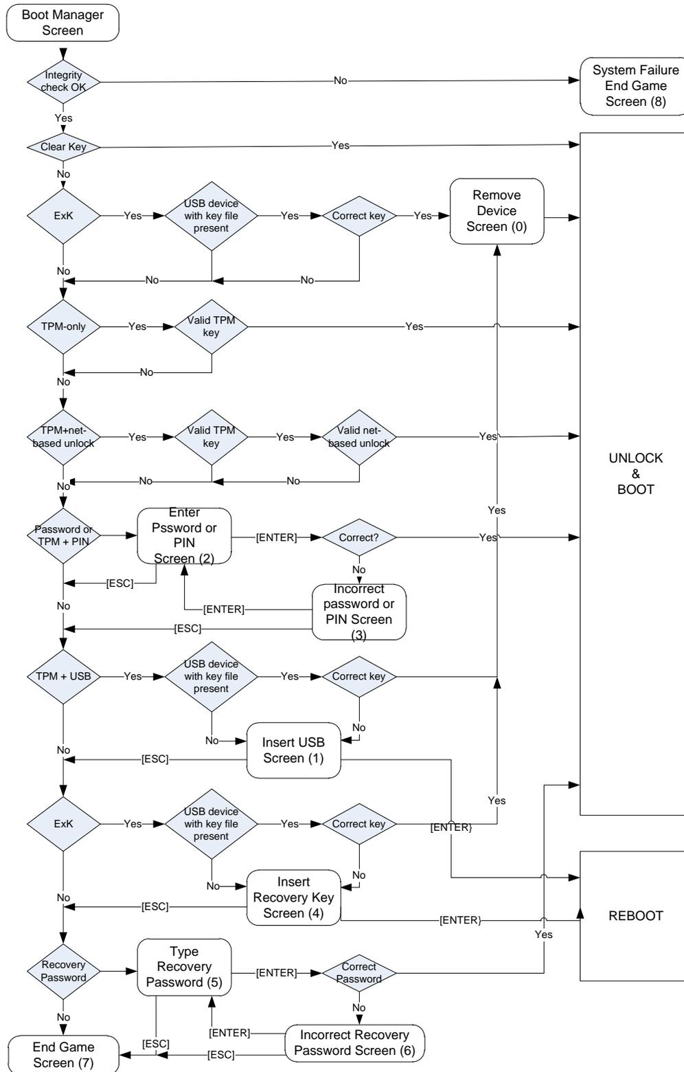
Figure 3 Flow Logic
