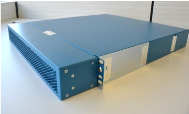
Figure 3 - PA-3060 Front Opacity Shield and Side
