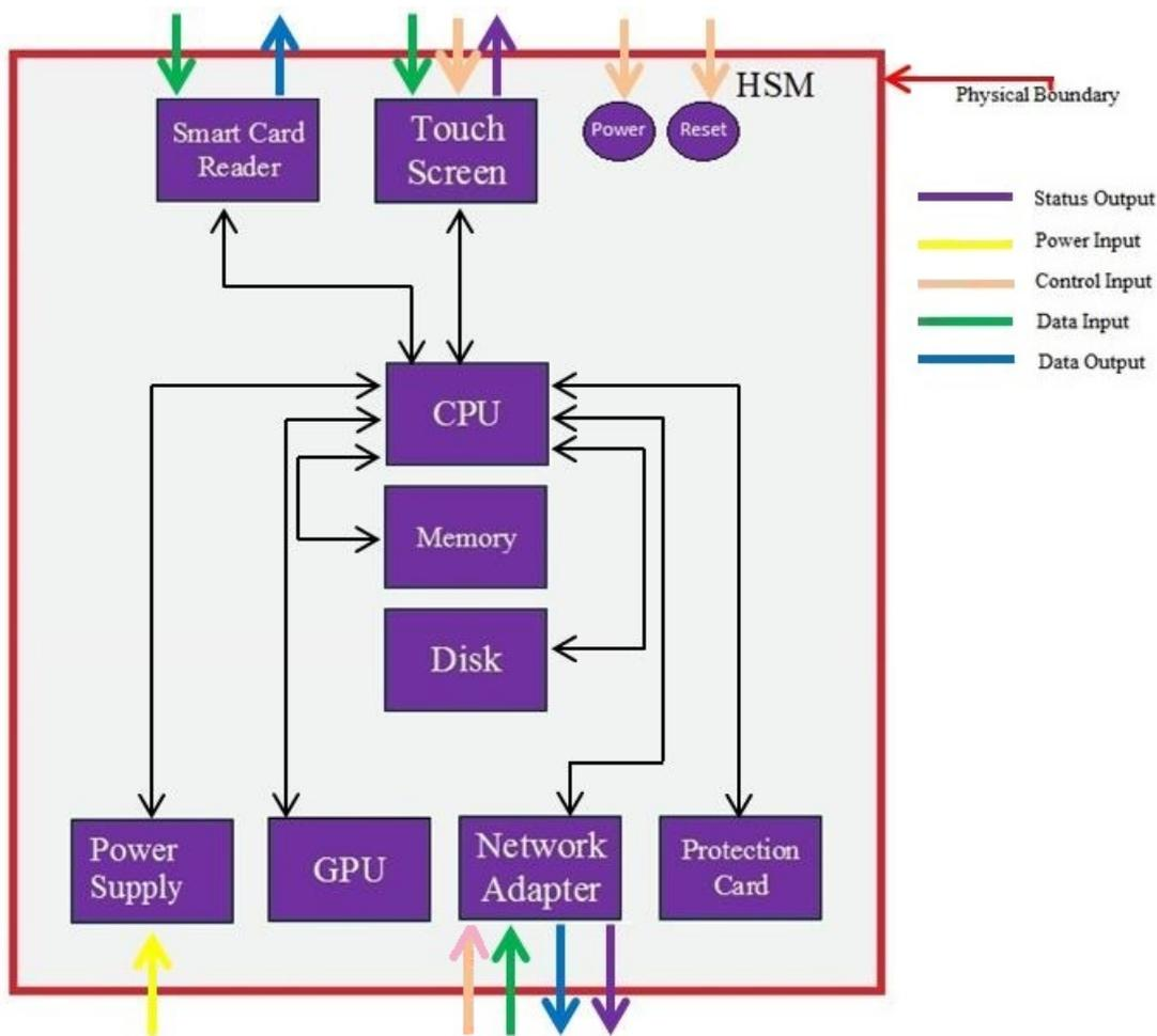
Figure 3: Hardware Block Diagram of HSM-ZJ2014
