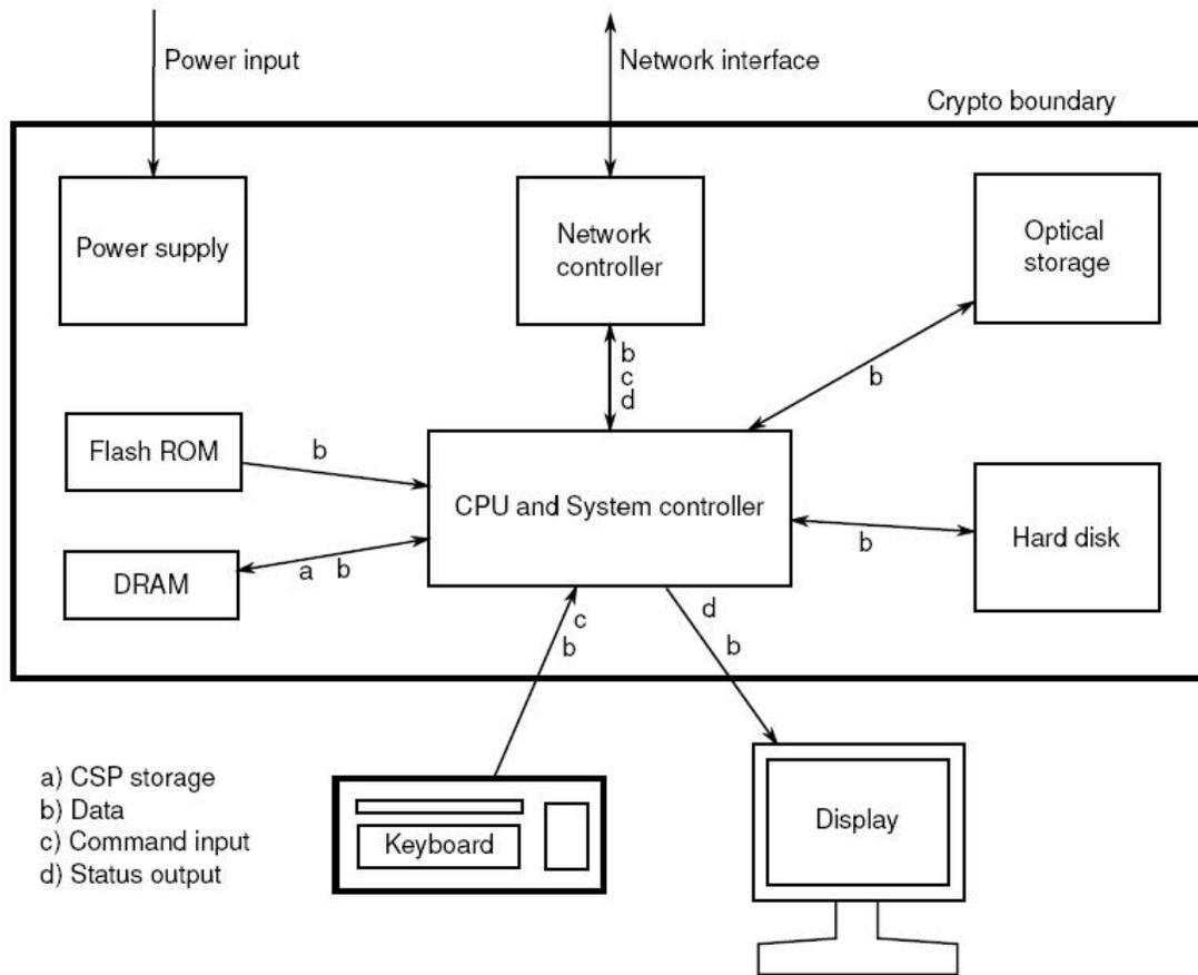
Figure 2 - Cryptographic Module Physical Boundary
