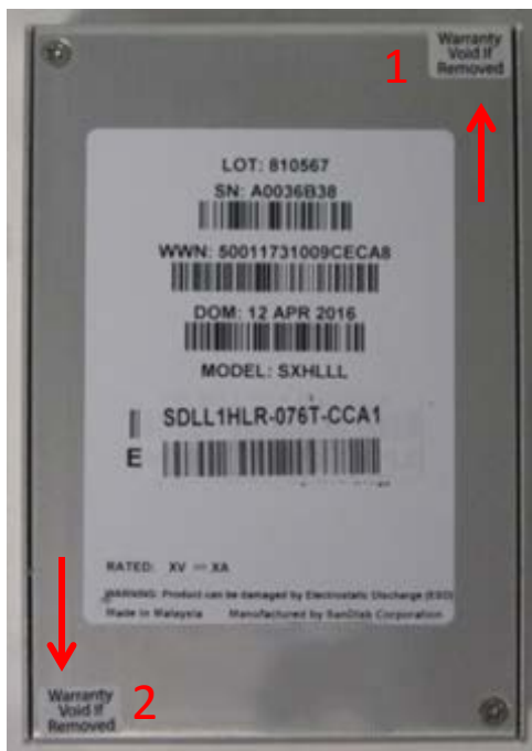
Figure 8. - Tamper-Evident Seal Location on Back Covering HDMI Port SDLL1HLR-076T Version 1 and SDLL1MLR-038T Version 1
