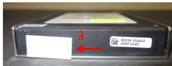
Figure 9 - Tamper-Evident Seal Location on Back Covering HDMI Port SDLL1CLR-020T Version 1 and SDLL1DLR-920G Version 1
