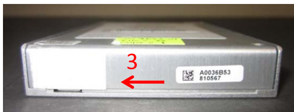
Figure 8. - Tamper-Evident Seal Location on Back Covering HDMI Port SDLL1HLR-076T Version 1 and SDLL1MLR-038T Version 1
