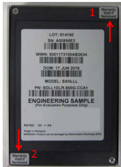
Figure 9 - Tamper-Evident Seal Location on Back Covering HDMI Port SDLL1CLR-020T Version 1 and SDLL1DLR-920G Version 1
