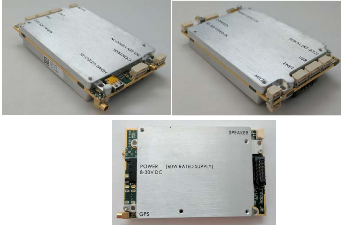
Figure 1 – Physical Boundary of Embedded Module
