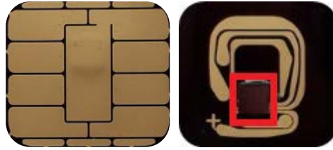
Figure 2 – Contact only interface: S-MFC6.8 front and back
