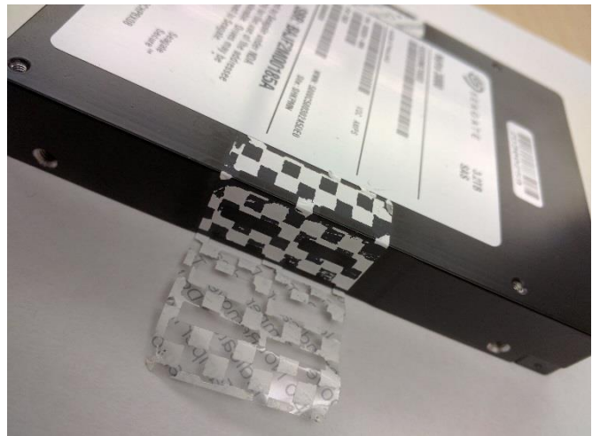
Figure 9: Nytro 3000® 15mm Label lifted
