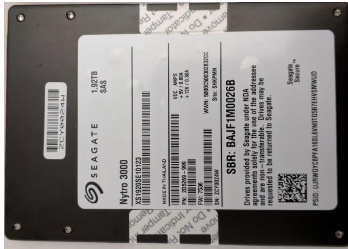
Figure 3: Top view of tamper-evidence label on sides of Nytro 3000® SAS Interface module
