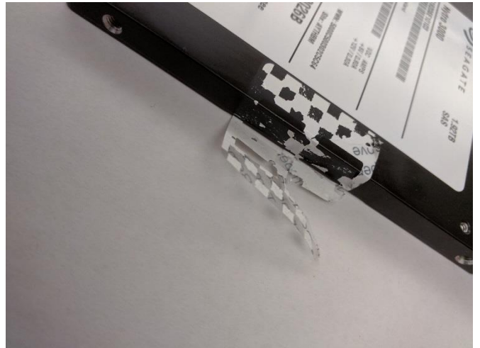
Figure 7: Nytro 3000® 7mm Label lifted off
