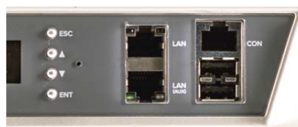
Figure 17 – RJ45 Ethernet, Console and USB close-up
