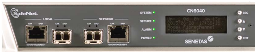
Figure 16 – A6040B [Y] 1G Ethernet / 1/2/4G Fibre Channel port close-up - SFPs installed
