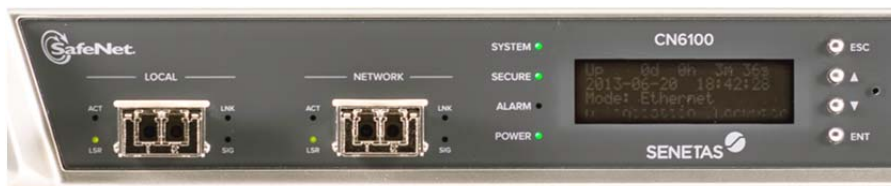
Figure 15 – A6100B [Y] 10G Ethernet port close-up - XFPs installed
