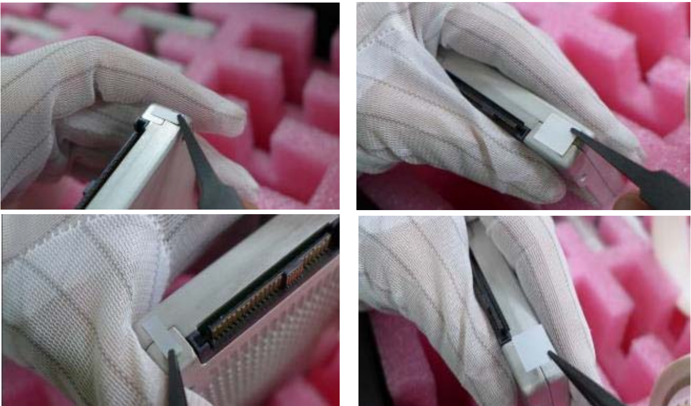
Figure 7 – Applying Tamper-Evident Seals
