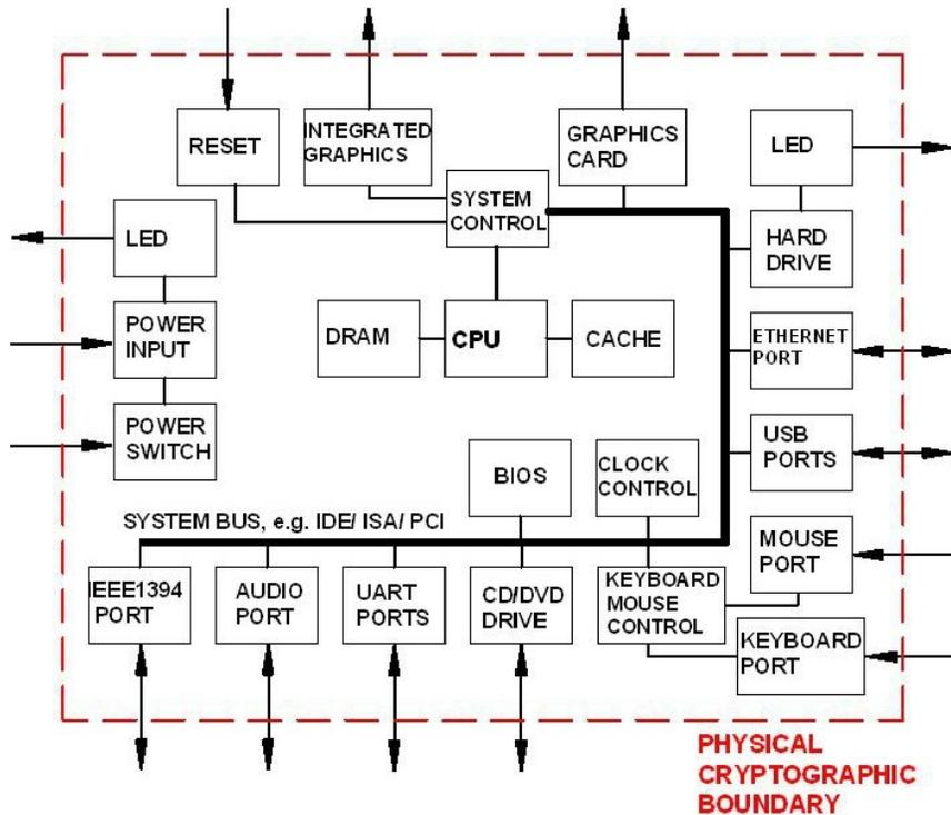
For FIPS 140-2 purposes, the BC-FJA Module is defined as a “multi-chip standalone module”, therefore, the module’s physical ports or interfaces are defined as those for the hardware of the GPC. These physical ports are separated into the logical interfaces defined by FIPS 140-2, as shown in Table 3.
