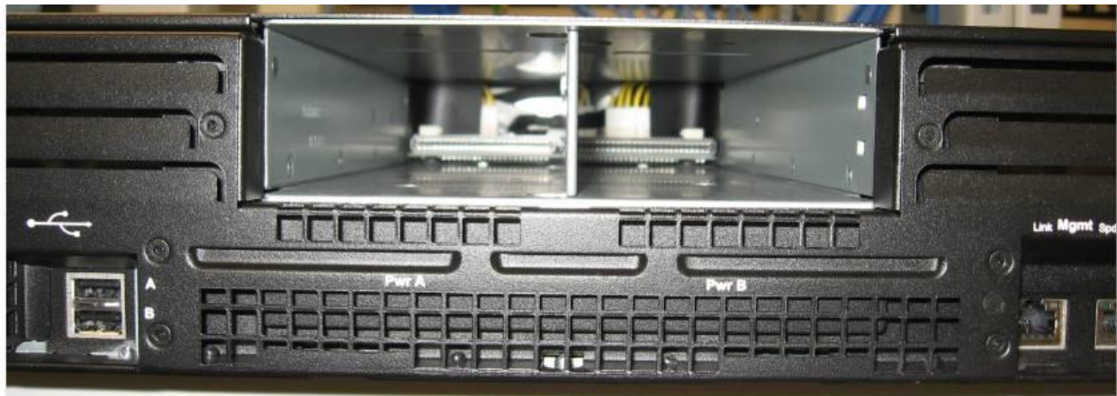
Figure 5 - Rear Panel with Power Supplies Removed
