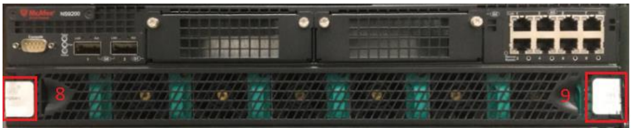
Figure 8 – Tamper Label Placement Front (NS9300 P sensor)
