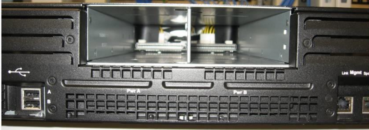
Figure 6 - Rear Panel with Power Supplies Removed
