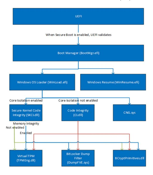
Boot Manager checks the integrity of the WINLOAD.EFI component of the Windows OS Loader before it is loaded.
