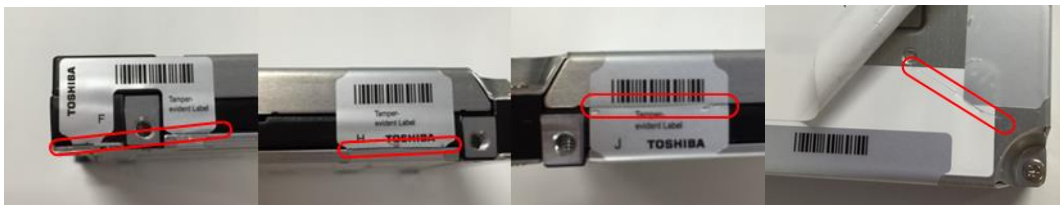
Figure 3 - Cutting line (Security seals and OUTER SHEET)
