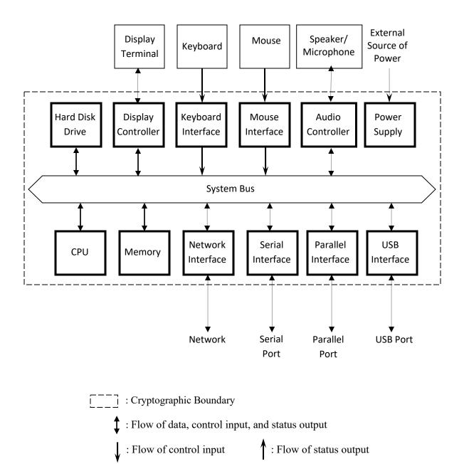
Figure 1: Cryptographic Module Hardware Block Diagram
