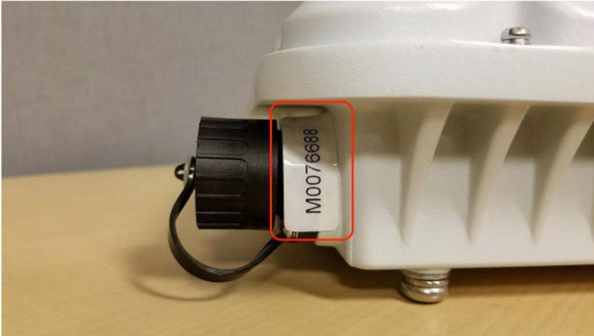
Figure 8: Tamper-evident seals on T710 Access Point
