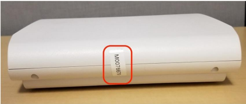
Figure 10: Tamper-evident seals on R710 Access Point
