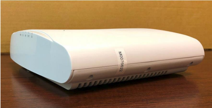
Figure 11: Tamper-evident seals on R720 Access Point
