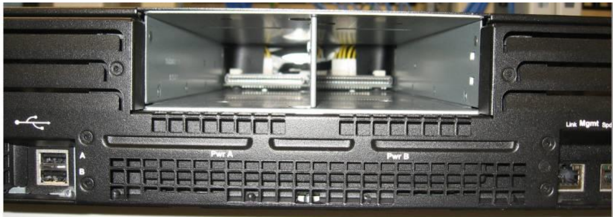
Figure 5 - Rear Panel with Power Supplies Removed
