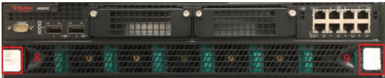
Figure 7 – Tamper Label Placement Front (9300 S)
