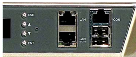
Figure 30 – CN6000 Series RJ45 Ethernet, Console and USB close-up
