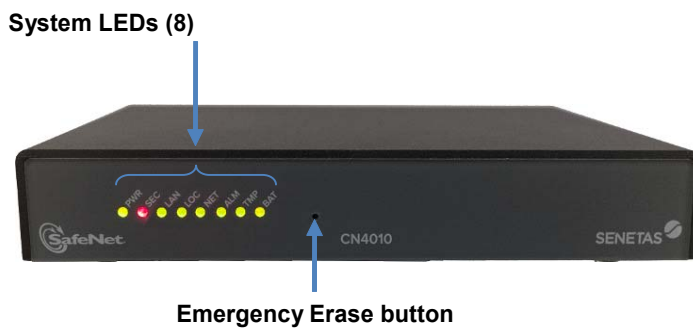
Figure 35 - Front View of the CN4010 Encryptor
