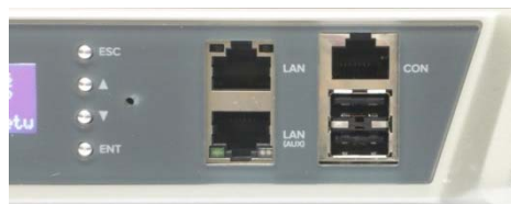
Figure 23 – CN9000 Series RJ45 Ethernet, Console and USB close-up
