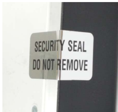
Figure 37 – CN9000 Series factory installed tamper seals
