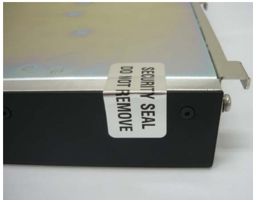
Figure 38 – CN6000 Series factory installed tamper seals
