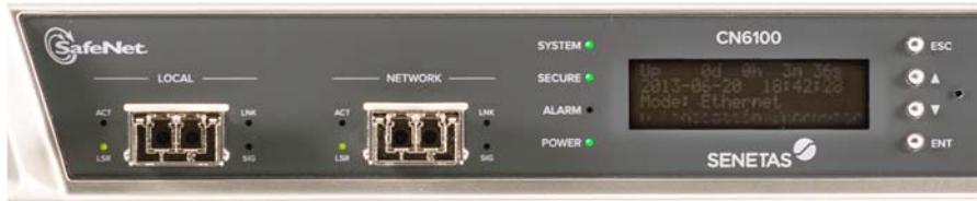
Figure 16 – A6100B [Y] 10G Ethernet port close-up - XFPs installed
