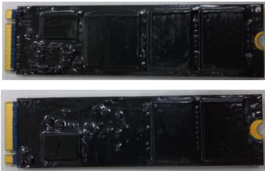
Exhibit 4 - *Specification of the DIGISTOR M.2 2280 NVME FIPS SSD Cryptographic Boundary (From top to bottom: top side, bottom side).*
