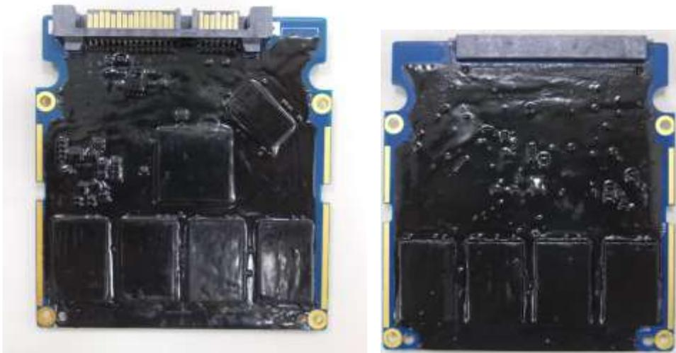
Exhibit 2- *Specification of the DIGISTOR 2.5-INCH SATA FIPS SSD Cryptographic Boundary (From left to right: top side, bottom side).*
