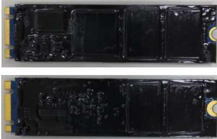
Exhibit 3 - *Specification of the DIGISTOR M.2 2280 SATA FIPS SSD Cryptographic Boundary (From top to bottom: top side, bottom side).*
