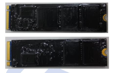
Exhibit 4 - Specification of the M.2 2280 NVMe NAND Flash SSD Cryptographic Boundary (From top to bottom: top side, bottom side).
