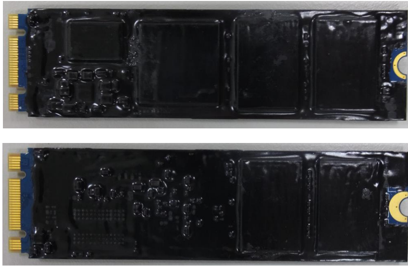
Exhibit 3 - Specification of the SQFlash 840F M.2 2280 SATA SSD Cryptographic Boundary (From top to bottom: top side, bottom side).
