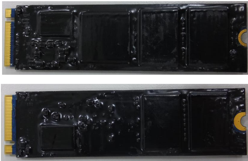
Exhibit 4 - Specification of the SQFlash 920F M.2 2280 NVMe SSD Cryptographic Boundary (From top to bottom: top side, bottom side).
