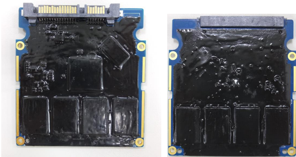
Exhibit 2 - Specification of the SQFlash 840F 2.5” SATA SSD Cryptographic Boundary (From left to right: top side, bottom side).
