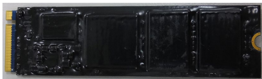
Exhibit 3 - Specification of the SQFlash 840F M.2 2280 SATA SSD Cryptographic Boundary (From top to bottom: top side, bottom side).
