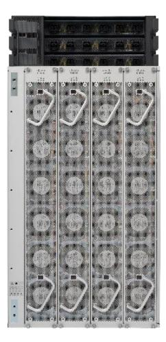
Figure 2: Rear View of Cisco 8800 Series Routers
