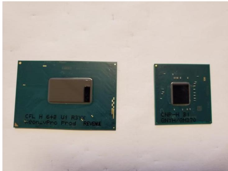
Figure 1b – Intel Cannon Point PCH with Coffee Lake (CFL) chipset
