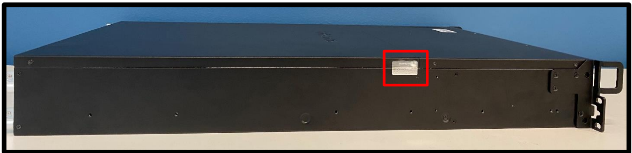
Figure 9. Tamper seal placement for NSsp 14700 and NSsp 15700 (Right)
