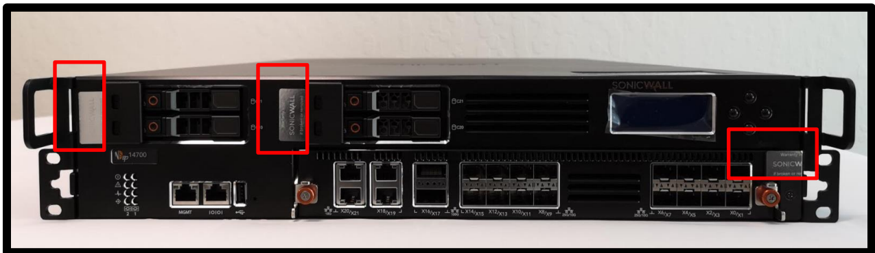
Figure 5. Tamper seal placement for NSsp 14700 (Front)
