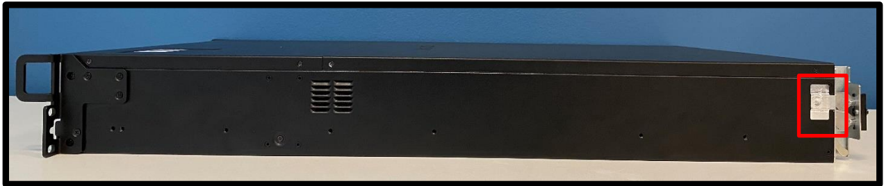
Figure 8. Tamper seal placement for NSsp 14700 and NSsp 15700 (Left)
