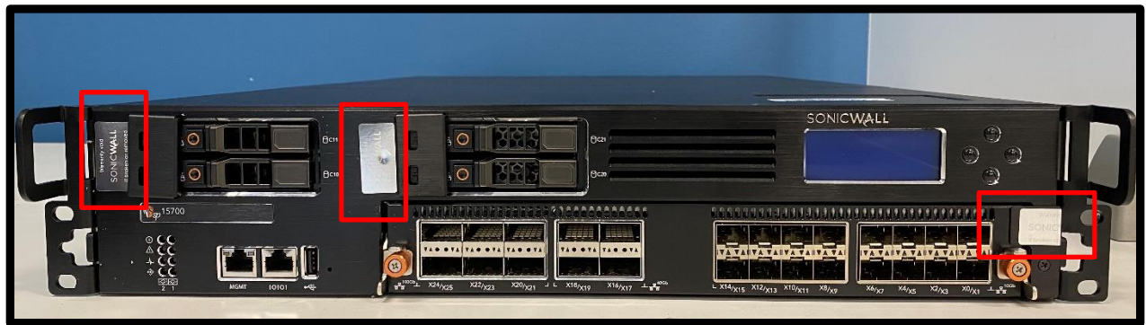
Figure 6. Tamper seal placement for NSsp 15700 (Front)
