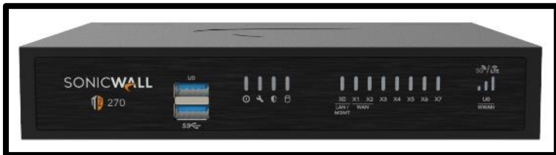
Figure 1. Front view of the physical ports on TZ270
