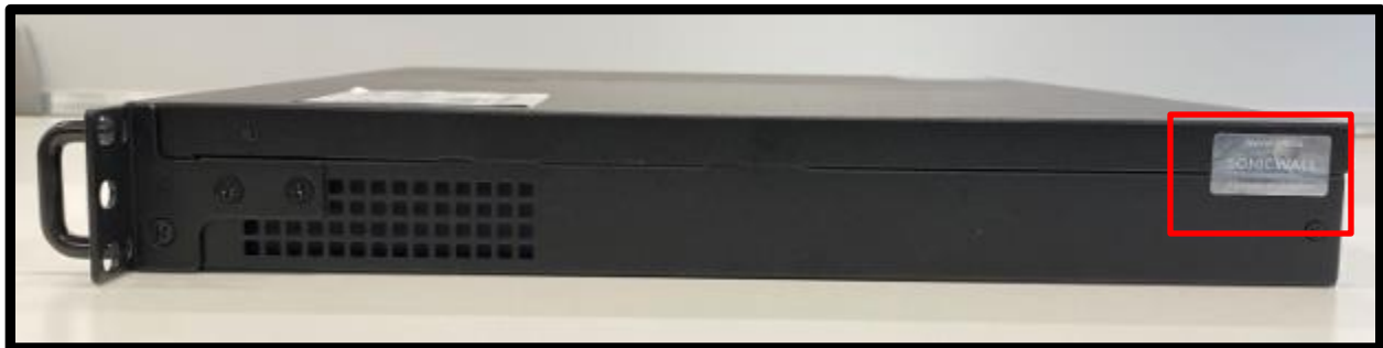
Figure 22. Tamper seal placement for NSa 2700/ NSa 3700 (Left View)
