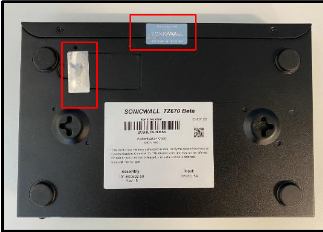
Figure 21. Tamper seal placements for TZ670 (Bottom View)
