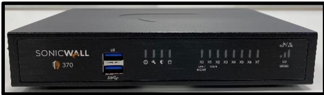
Figure 3. Front view of the physical ports on TZ370
