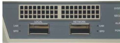
Figure 22 – A9120B 100G Ethernet ports close-up – QSFP28s not installed
