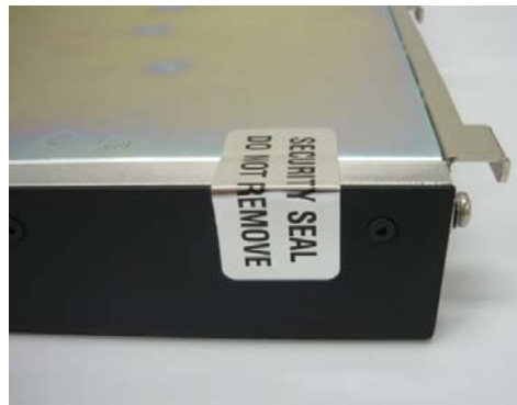
Figure 38 – CN6000 Series factory installed tamper seals
