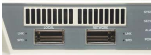
Figure 21 – A9100B 100G Ethernet ports close-up - CFP4s not installed
