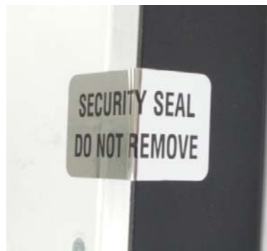
Figure 37 – CN9000 Series factory installed tamper seals
