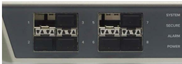
Figure 27 – A6140B Ethernet port close-up - SFPs not installed
