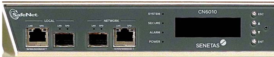
Figure 29 – A6010B 1G Ethernet port close-up - SFPs not installed
