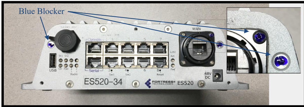
Figure 6 ES520 Version 2 (Front) Tamper Evidence (3 screws)
