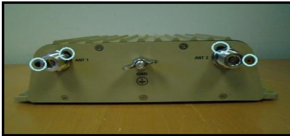
Figure 5 ES520 Version 1 (Rear) Tamper Evidence (4 screws)
