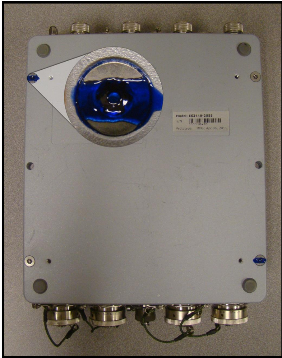
Figure 2: ES2440 Tamper Evidence (2 screws)
