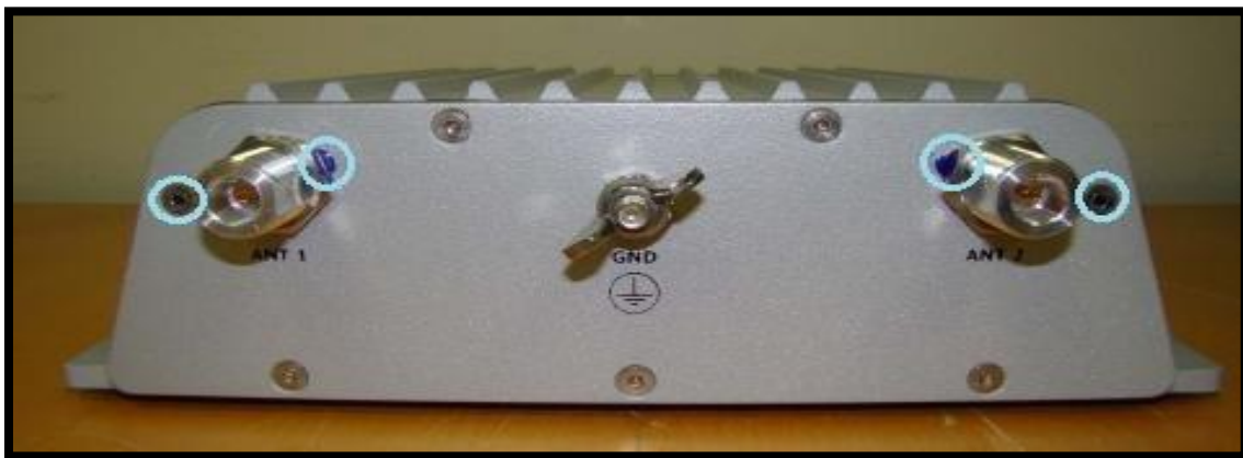
Figure 7 ES520 Version 2 (Rear) Tamper Evidence (4 screws)
