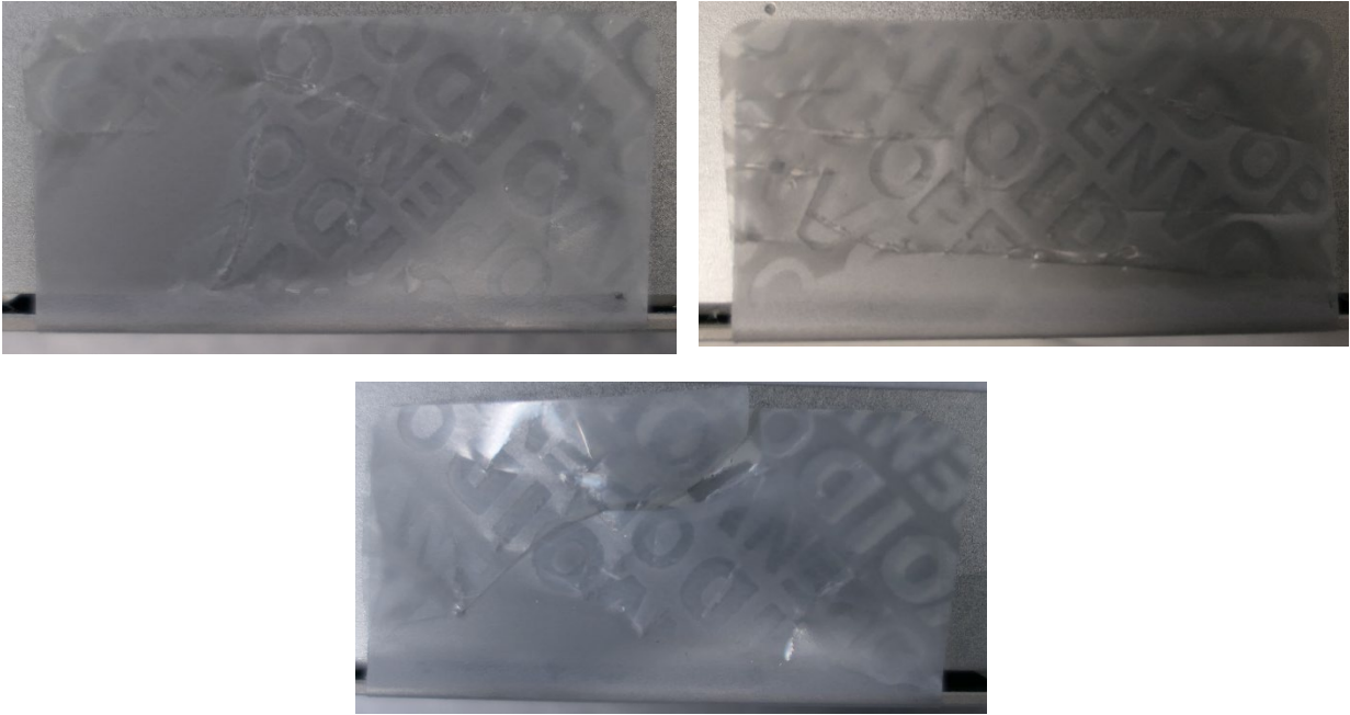
Figure 4: PE8000 Series NVMe OPAL SEDs Tamper Evidence
