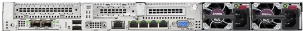
Figure 3 – IPsec IPGW Rear Panel
